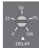
If using digital servo, please set delay time trimmer to the position of "0" while using normal servo, please adjust the delay volume according to the detailed fact.
