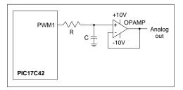
Choosing, the -3 dB point at 4 KHz, and using the relation RC = 1/(2\* $\pi$ \*f), we get R = 4 K $\Omega$ , if C is chosen as 0.01  $\mu$ F :
